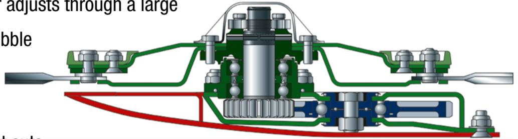
blockage-free and clean. Benefitting from massive double spur gear bearings that are spaced at large gaps, the cutterbars are heavy-duty and hardwearing.
