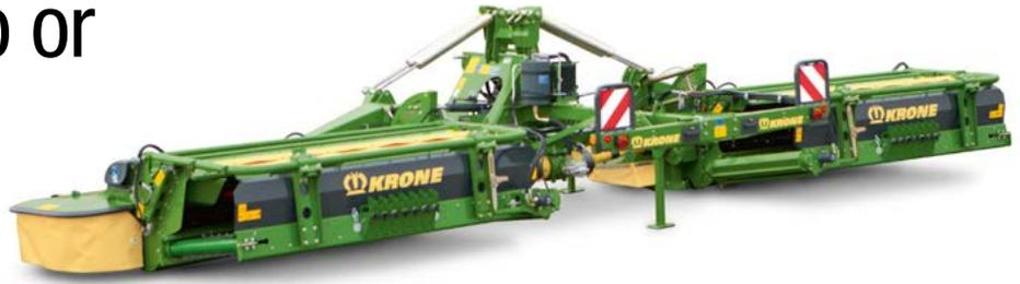
The Collect cross conveyor belts make very versatile machines of the EasyCut B 870 CV and B 1000 CV with steel tine conditioner, and the EasyCut B 870 CR and B 1000 CR with roller conditioner, allowing the units to spread the material or present it in a single swath. The powerful belts handle even the heaviest crop most effectively, lifting and lowering hydraulically either in sync or independently. Each belt itself is shut off automatically when the unit lifts out of work.
