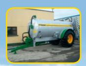
2250 galvanized with 7 meter trailing shoe
