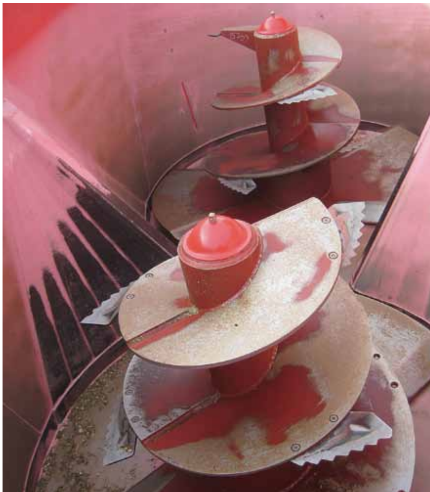
Figure 3: The vertical mixing augers of the Trioliet Solomix 2-2000 VLH-B feed-mixer wagon
